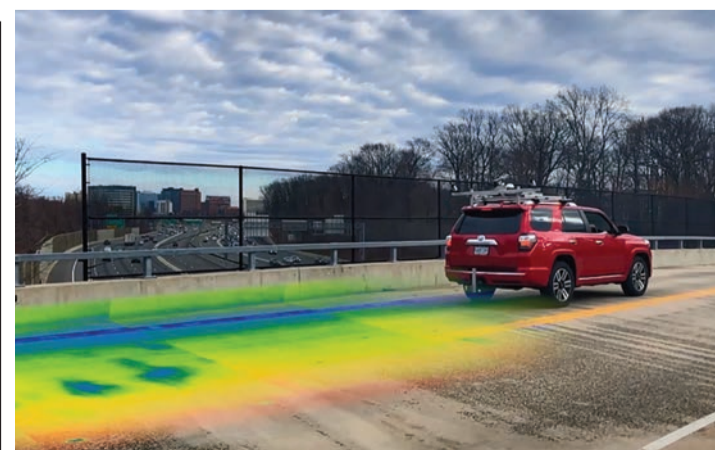
West Nippon Expressway's thermography technology allows engineers to determine the true condition of roads in need of maintenance.
